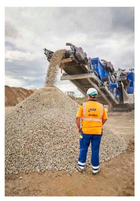
We recycle non-hazardous and surplus worksite waste (concrete, ballast, asphalt, excavated earth and spoil).
